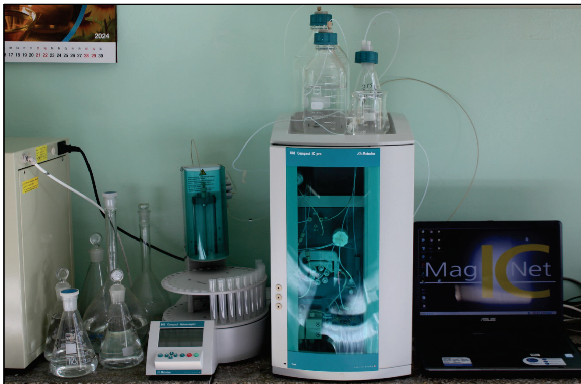
Fig. 1. Ion chromatograph Compact IC PRO 881 Metrohm with conductometric detector (range 0–15,000 \mu\text{S}/\text{cm} , Switzerland; Institute of Plant Physiology and Genetics, NAS of Ukraine); determination of the amount of inorganic anions and cations in plants was carried out on a Metrosep A Supp 5,250x4.0 mm column, eluent – carbonate buffer 3.2 mM Na 2 CO 3 + 1.0 mM NaHCO 3 for determination of anion content and a Metrosep C2 150x4.0 mm column, eluent – nitric acid (50 mM) for determination of cation content (Merck reagents, Germany); plants were divided into separate organs, dried, and homogenized; each individual 50 mg plant material was dissolved in 10 mL (for anion determination) and 15 mL (for cation determination) of ultrapure water of class 1 (Ultra Pure Water System, Human Corporation, Korea/Left block) and extracted in a boiling water bath for 10 min, the extract was collected and repeated under the previous conditions three times; the total amount of water was 50 mL (1:1000 dilution) for cationic content and 30 mL (1:600 dilution) for anionic content; the extract was filtered (0.22 or 0.45 nm); primary data processing was performed using the Magic Net IC v. 1.1 program by Metrohm (Switzerland)
